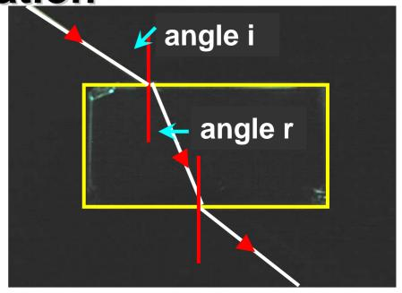
3. Shine rays of light with incident [i] angles of 30°, 60° and 0° into the block, making sure they all hit where the normal line crosses the glass surface.
