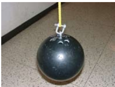
Attach the ball securely to the braided rope with a U-bolt.
