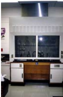
A fume hood designed for wheelchair
