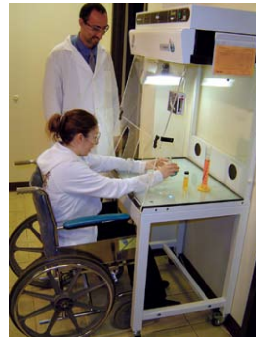
Ductless fume hood accessible to student in wheelchair
