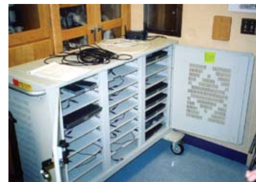
A laptop computer storage and recharging cart
